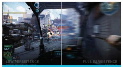
VR displays pulse on and off very rapidly for 'low persistence' to reduce blurring. OLEDs are great for this, and MicroLEDs will be even better
